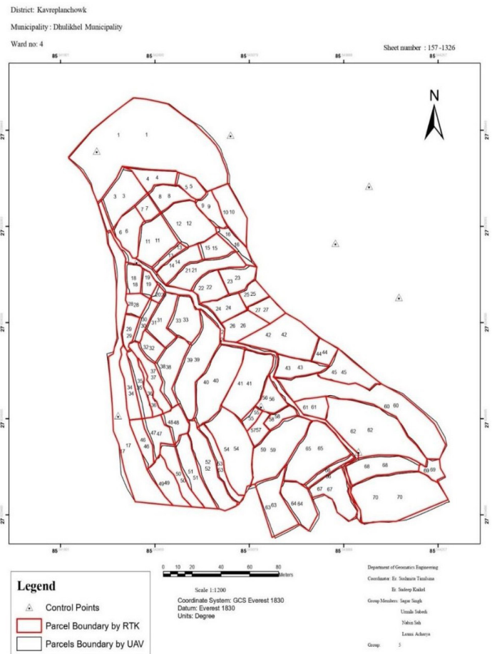
Figure 7: Overlapping area of RTK-GNSS and UAV Cadastral Map
