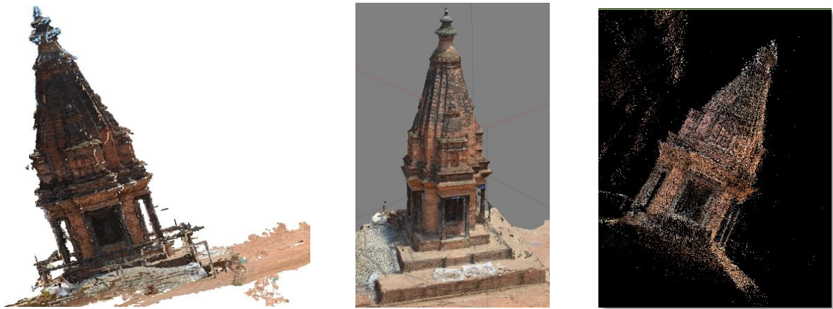
Fig 3: Textured Model generated from NIKON images using VisualSFM (left), Agisoft PhotoScan (middle) and point cloud generated from Microsoft Photosynth (right)
