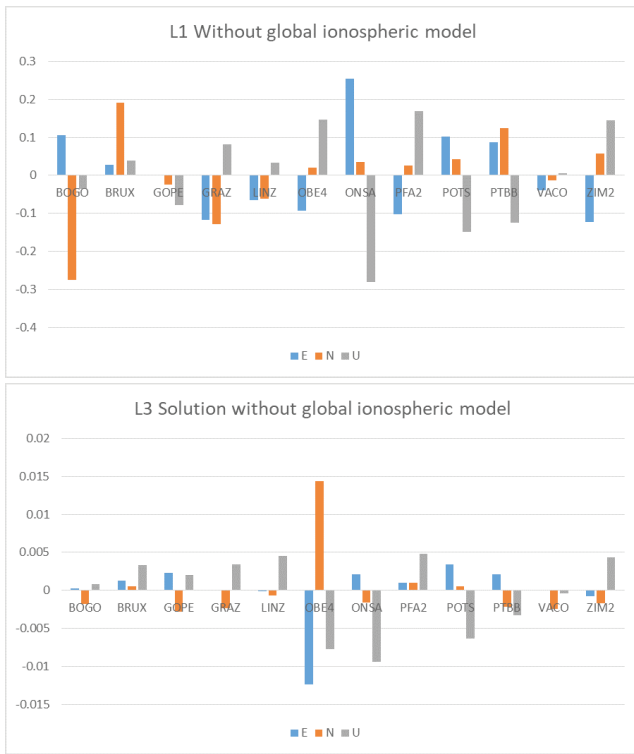
Fig 2: Residue in station coordinate while using L1 and frequency and no ionospheric model Fig 3: Residue in station coordinate while using L3 and frequency and no ionospheric model
