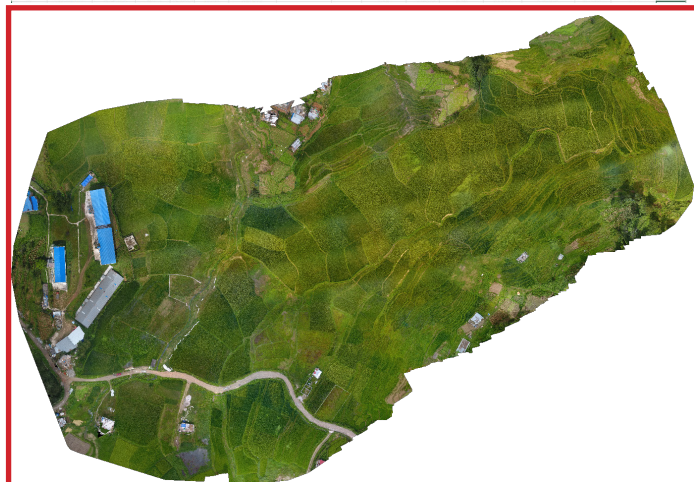
Figure 5 Merged aerial photographs of study area with image resolution 24733 x 16975(280 images merged)
